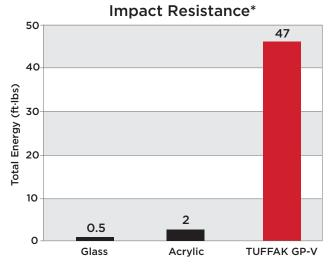
\*Instrumented Impact per ASTM D 3763, sample thickness 0.125" nominal
