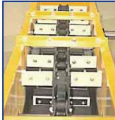
Grain drag flights manufactured from TIVAR® H.O.T. last longer and perform better in higher temperatures or where chemicals such as Hexane are used than those manufactured from standard UHMW.
