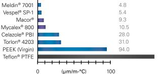
The coefficient of linear thermal expansion is the ratio of the change in length per degree C to the length between 23 °C and 250 °C. Per test method ASTM E-831.
