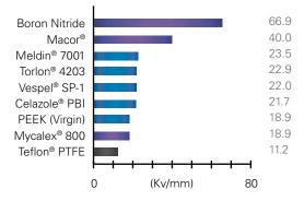
The maximum voltage that can be applied to a given material without causingit to break down,usually expressed in volts or kilovolts per unit of thickness.
