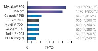
The maximum acceptable temperature above which mechanical properties (tensile strength, impact strength) or electrical properties (dielectric strength, linked to insulation properties) of a part are significantly degrading, over the reasonable life time of the tested product.
