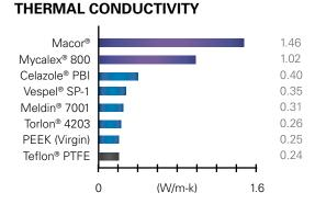
Thermal conductivity is the quantity of heat transmitted through a unit thickness in a direction normal to a surface of unit area, due to a unit temperature gradient under steady state conditions.
