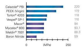
Measure of the ability of rigid plastics to withstand permanent deformation and the ability of non-rigid plastics to return to original shape after deformation. Standard test methods for determining both types of deformation under load are given in ASTM D-621.
