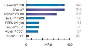
Maximum stress a material can sustain under crush loading. The compressive strength of a material that fails by shattering fracture can be defined within fairly narrow limits as an independent property. However, the compressive strength of materials that do not shatter in compression must be defined as the amount of stress required to distort the material an arbitrary amount.
