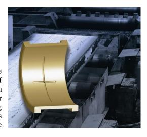
The BR60 and BR70 laminates consist of multiple piles of heavy-weight canvas cloth saturated with phenolic resin system, modified disulfide, which provides internal lubrication to reduce frictional heat generation and wear of metal shafts on the bearing. The pre-preg piles are then laminated under heat and pressure to produce the thermoset composite material.
