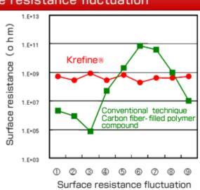
As illustrated in the graph above, Krefine's new technology results in consistent and controlled surface resistance for each point at specific levels within the range of 10<sup>6</sup> to 10<sup>11</sup> ohm on an injection molded specimen. The surface resistance of a carbon fiber reinforced compound however, is highly variable versus that of the Krefine molded part. This variability is due to uneven distribution of the carbon fiber at the parts
