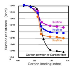
Beyond a certain critical special carbon content, the surface resistance of a compound decreases with an increase in the special carbon content to 10<sup>10</sup> ohms. The surface resistance of the compound in the critical
