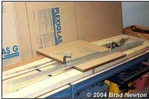
When routing a long piece it's a good idea to brace your straight edge in the middle as shown to prevent any bowing along the way.
