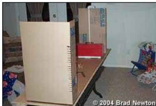
Once the sides are seamed to the back panel, wait 4 hours and flip the tank over (carefully, with a helper) and seam the sides to the front. Notice the jig is now used to hold the center of the back panel from sagging. Just remove the two PVC elbows and it's the perfect height.
