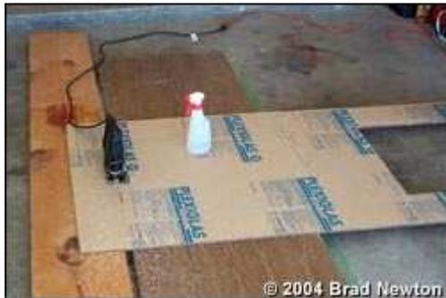
If you have any internal integrated overflows, here's a good way to make your overflow teeth. I use a 1/4" straight cut router bit and a couple straight edges. Here's the setup. It allows for exact depth control and I like to keep 1/2" of acrylic between each notch and go down 1.25" into the sheet.
