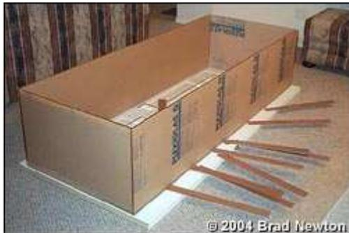
Wait 4 hours, flip the tank over and seam the bottom
