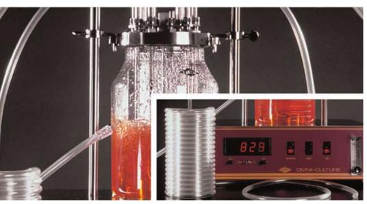
Clear and flexible, TYGON® 2475 High Purity Tubing is ideally suited for use in many sensitive cell culture and fermentation applications.
