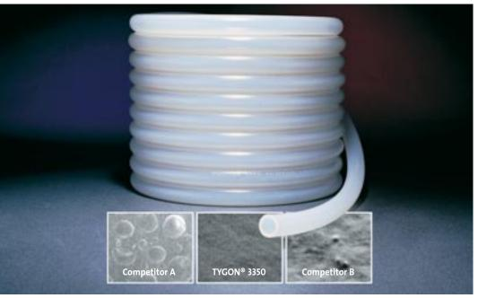
In a comparison of images of the inner surfaces of TYGON® 3350 silicone tubing and two competitors (captured at 500 x magnification with an electron scanning microscope), TYGON clearly exhibits superior smoothness. As a result, potential for particle entrapment is greatly reduced.
