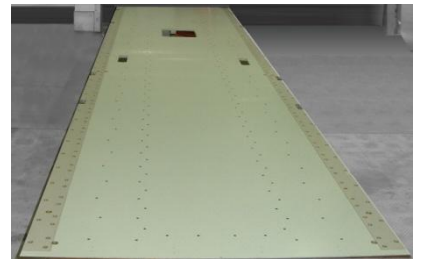
Pre-finished roof panel including fixation points for infrastructure and protection against burn-in from sparks (Dimensions: 2.41 x 10.34 m)
