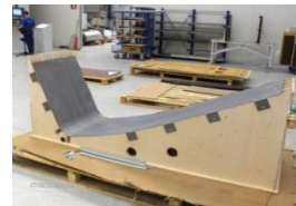
Sandwich part tool for oven curing at 135°C
