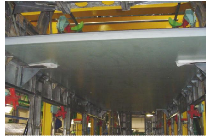
Double deck wagon with self-supported intermediate floor (2.64 x 8.09 m), steel construction
