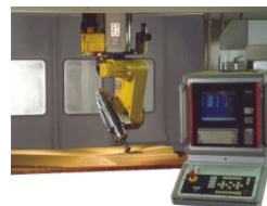
Machining of honeycomb
