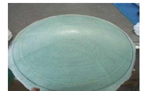
Tool produced with RI for the contouring of formed honeycomb core details
