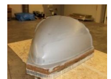
Finished mold after final milling
