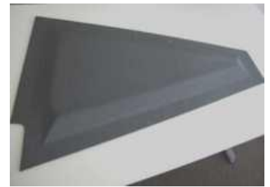
Structural part with honeycomb core and carbon skins
