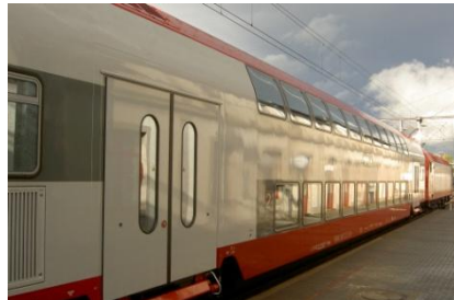
Double deck wagon with self-supported intermediate floor (2.61 x 15.46 m), aluminum construction
