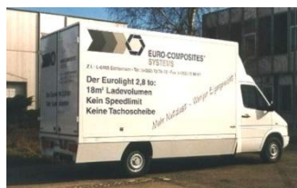
Panels up to 15,0 m length for truck superstructures
