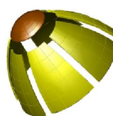
Radome made from formed honeycomb core details
