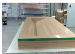
Coated PU tool for model making
