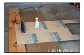
If you have any internal integrated overflows, here's a good way to make your overflow teeth. I use a 1/4" straight cut router bit and a couple straight edges. Here's the setup. It allows for exact depth control and I like to keep  $\frac{1}{2}$ " of acrylic between each notch and go down 1.25" into the sheet.
