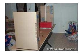
Once the sides are seamed to the back panel, wait 4 hours and flip the tank over (carefully, with a helper) and seam the sides to the front. Notice the jig is now used to hold the center of the back panel from sagging. Just remove the two PVC elbows and it's the perfect height.
