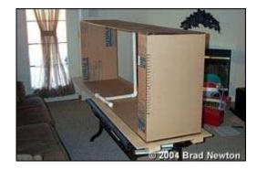
Wait 4 hours, put the assembed sides on the top panel and seam. Note the use of shims in this pic.
