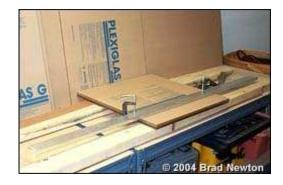
When routing a long piece it's a good idea to brace your straight edge in the middle as shown to prevent any bowing along the way.
