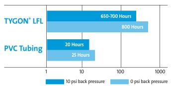
The performance of tubing in peristaltic pumping applications is affected by the conditions of use and equipment utilized, along with size and wall thickness of the tubing tested. The data above is presented for information only and should not be utilized for specification purposes.
