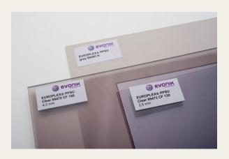
coating (DF). Functional coating for EUROPLEX® PPSU transparent sheet provide hardness, nonglare light-scattering surfaces combined with improved climatic resistance.
