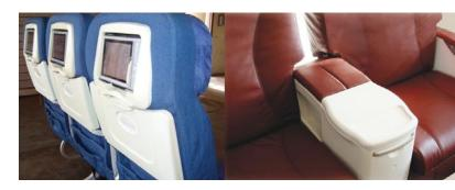
thermoformed aircraft interior components.
